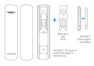
5.2 Install the fastening clip SmartBracket on the door frame and door or window frame and window with a help of the expansion bolts and self-tapping screws included in the set. 5.3 Put the sensor on the SmartBracket. Once the sensor is fixed on the SmartBracket, its light must blink. It means that the tamper on the sensor is shut. In case the sensor does not blink, the tamper status must be checked at the receiver configuration software!
