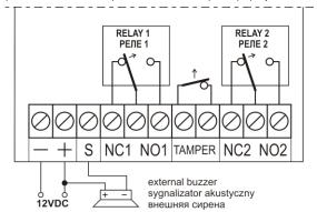
IMPORTANT! Output S must not be directly connected to (+) pole of power supply (see
