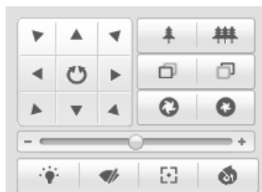
Figure 4-4 Panou de control PTZ
