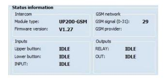
Displays information about the switching state of the peripheries and the actual status of the mobile network.
