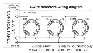
Base terminals "1" and "2" for DC power input, non-polarized. "4" for DC power anode or cathode output. "3" for relay output COM. "4" for relay output N.C. or N.O..
