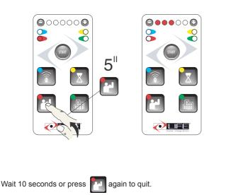
Press for 5 seconds, the red LED (SX) will light and then switch off.
