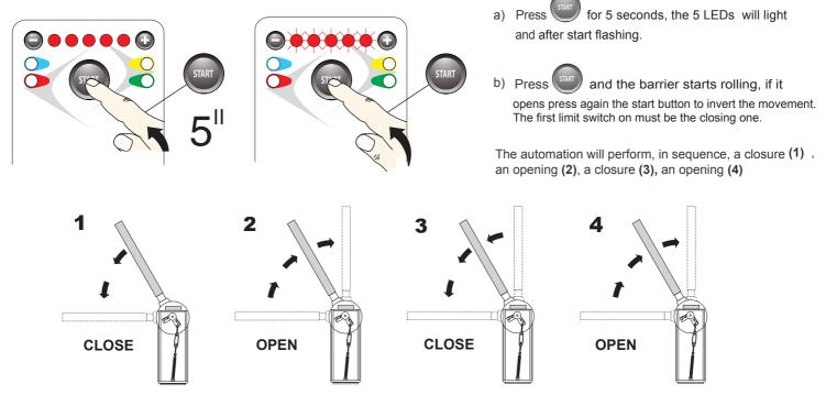
Once programming is complete, the two green LEDs will Flash and the red one will be fix. Should the result obtained not be satisfactory, repeat the whole process.
