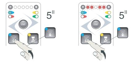
a) Press limit the radio icon button (top left) for 5 seconds.
