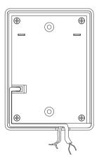
4. If there is no hole on the wall, you can allocate the wire on the groove around the case as appeared in the figure.
